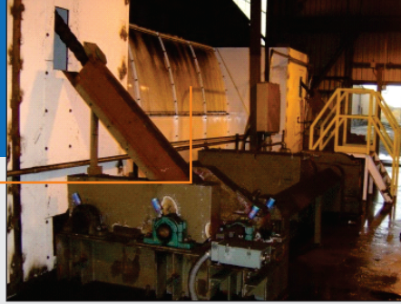
'Contoured Enclosure' ensuring containment of Fog and Dust
