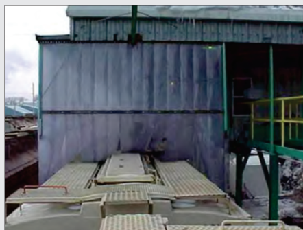
Flexible Enclosure in loading application
