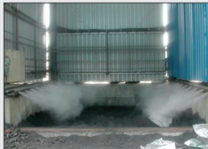
Containment in Dump Hopper Application
